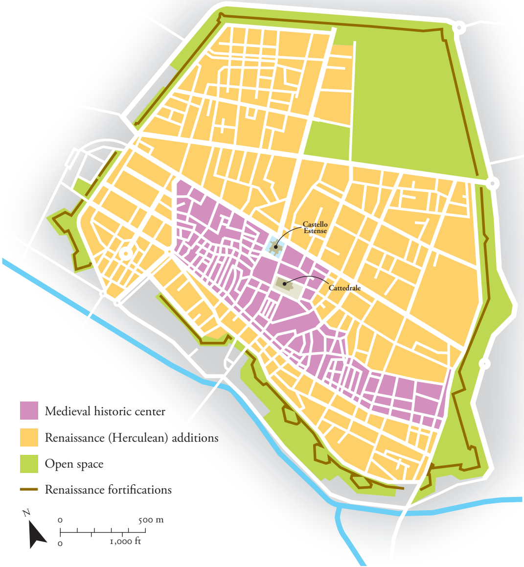
Map 9.4 The Urban Plan of Ferrara. The first successful example of Renaissance town planning, Ferrara has been designated a World Heritage site. The plan was the vision of Duke Ercole d'Este, who saw the need for a new, modern quarter to allow for a larger population. The medieval center of Ferrara is shaded in lilac on the map; around it, in gold, lie the straight, wide streets and the massive new walls (in brown). This area was named in honor of the duke: addizione erculea (Herculean Addition). Architect Biagio Rossetti (c. 1477–1516) designed the area according to Renaissance humanist principles, with palaces and other structures powerfully reflecting the influence of ancient building.
